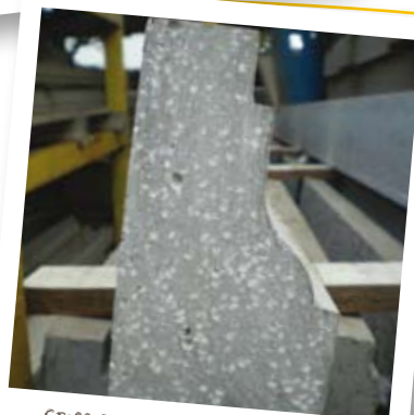
Cross section of concrete products showing the blended polystyrene
